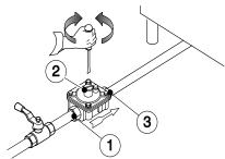
**NOTE!** These models are designed and certified for use with natural or propane gas. For natural gas, the pressure regulator on the header is set to 8" w.c. (20mbar).
